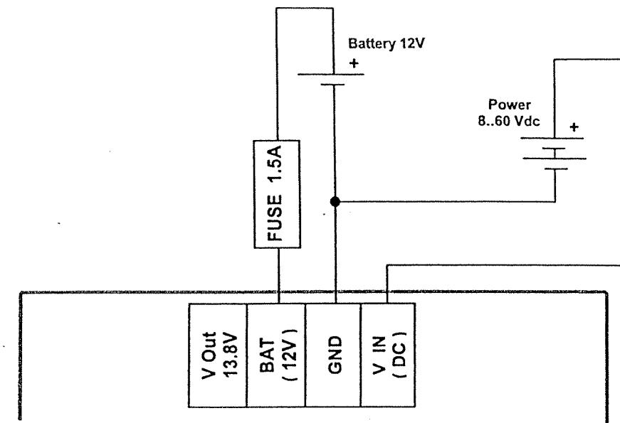
■ A Battery connection to a Booster must **absolutely be protected by a FUSE (1.5 A)**
