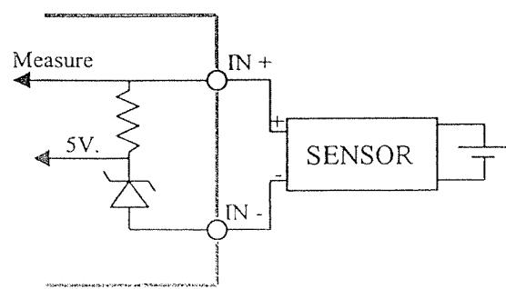
The current of the loop is used to power the input circuit with the help of the Zener diode.
