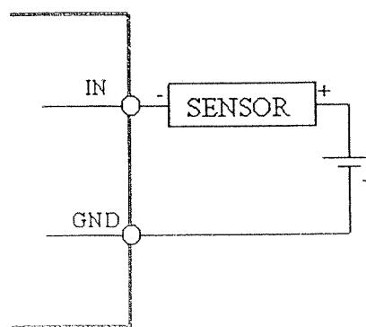
With this cabling you have to check the voltage needed by the Sensor.
