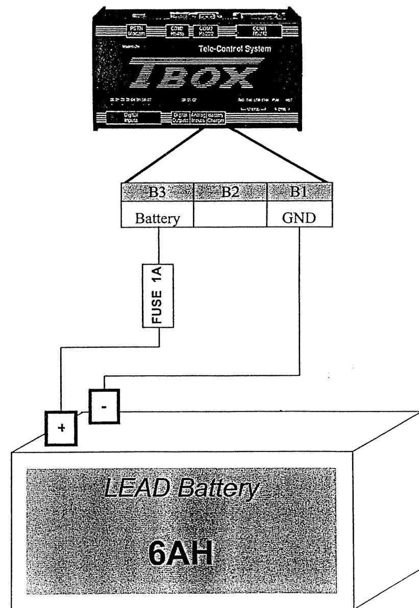
**CAUTION :** The '+' of the battery must be protected by an external 1 A fuse.
