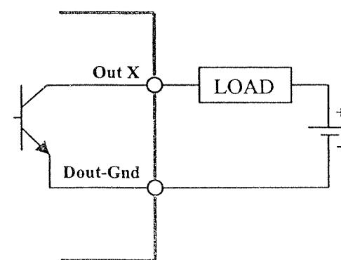
□ GND is common to the three outputs and isolated from the 0V. of the CPU.
