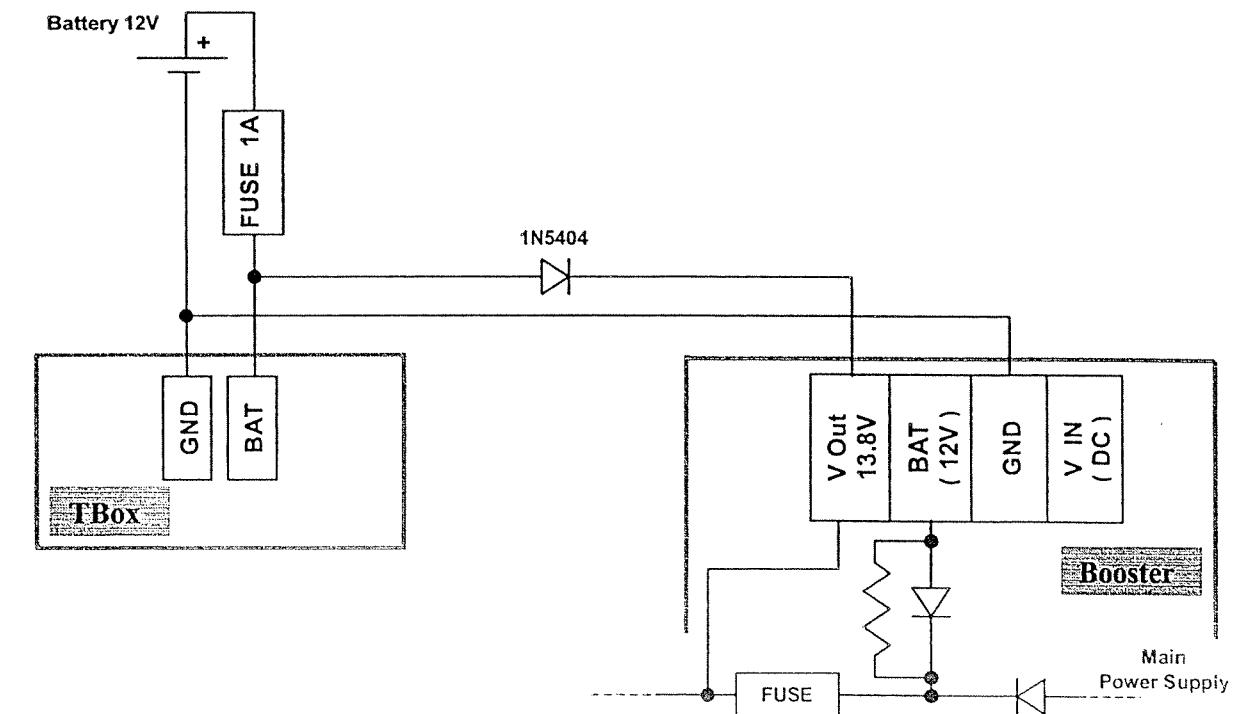
■ If an external battery of a TBox is used as back-up voltage for a Booster, it must be connected through a **diode** in serie as explained in the schematic. The internal circuit of the Booster explains the reason of cabling to 'V Out'.
