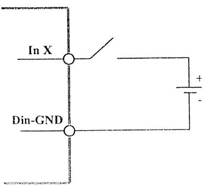
■ GND is common to the eight inputs and isolated from the 0V. of the CPU.
