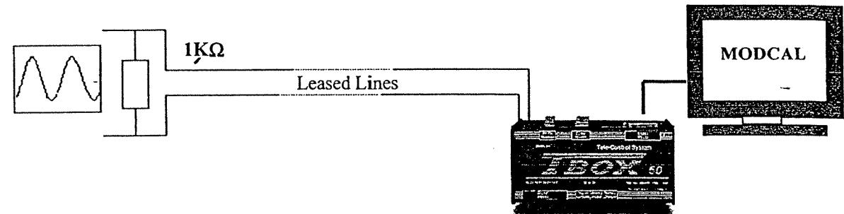
Adjust the potentiometer of the Network modem, indicated "LEVEL" on the CPU, beneath the connector of the digital inputs. This potentiometer adjusts the level of transmission. You must obtain a 1V peak to peak signal at the other end.
