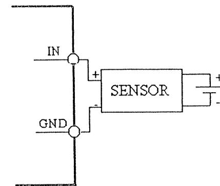
■ GND is common to the two inputs and to the power of the CPU.
