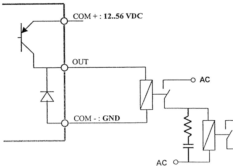
■ The output is protected by an internal diode. It is **indispensable** to protect the secondary relay with a RC (in case of AC relay) or with a diode (in case of DC relay) otherwise, it can affect the output stage of the card.
